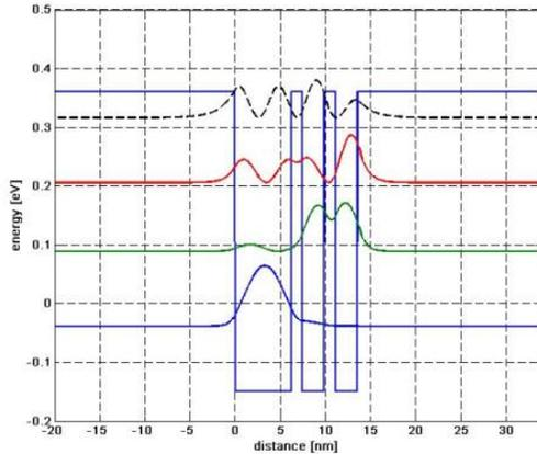
Figure 3. The lowest four electron envelope functions moduli squared and the corresponding eigen energies of an  $\text{Al}_{0.48}\text{In}_{0.52}\text{As}/\text{In}_{0.53}\text{Ga}_{0.47}\text{As}$  triple quantum well structure produced by MQWSS.
