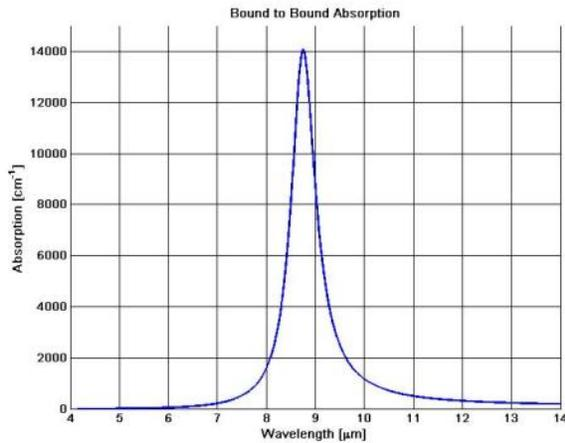
Figure 5. Absorption spectra (intersubband transition) for an  $(\text{In}_{0.53}\text{Ga}_{0.47}\text{As})_{0.15}(\text{InP})_{0.85}/\text{In}_{0.53}\text{Ga}_{0.47}\text{As}/(\text{In}_{0.53}\text{Ga}_{0.47}\text{As})_{0.55}(\text{InP})_{0.452}$  asymmetric step quantum wells structure produced by MQWSS.
