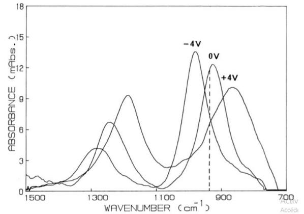
Figure 7. Measured Bound to Bound absorbance for 1-2 and 1-3 transitions in asymmetric step quantum wells structure at different voltage from [21].
