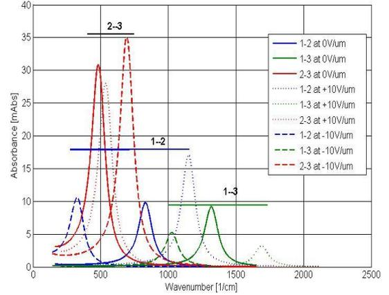
Figure 6. Bound-to-bound absorbance for 1-2, 1-3 and 2-3 transitions in asymmetric step quantum wells structure at different applied electric field produced by MQWSS.
