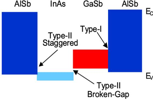
Figure 2. Schematic representation of the band alignments in the nearly matched InAs/GaSb/AlSb material system. The solid rectangles indicate the relative position of energy gaps and band edges of the different material among each other [8], [9].
