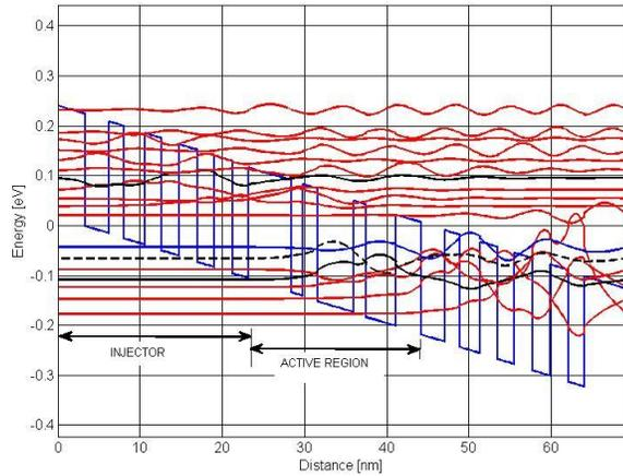
Figure 8. Band edge structure of a GaAs/AlGaAs QCL laser under an applied electric field of 48 kV/cm. The wavy curves are the wave functions. The transition states of active region are black, dashed black and black from bottom to top respectively.
