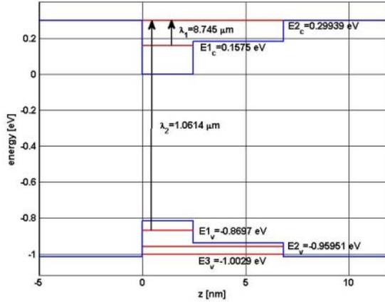
Figure 4. The lowest two electron eigen energies for an  $(\text{In}_{0.53}\text{Ga}_{0.47}\text{As})_{0.15}(\text{InP})_{0.85}/\text{In}_{0.53}\text{Ga}_{0.47}\text{As}/(\text{In}_{0.53}\text{Ga}_{0.47}\text{As})_{0.55}(\text{InP})_{0.452}$  asymmetric step quantum wells structure produced by our simulator.
