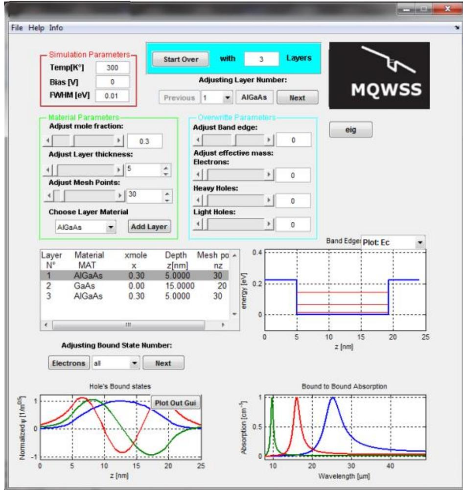
Figure 1. The main MQWSS user interface with a set of instructions implementing an AlGaAs/GaAs/AlGaAs heterostructure.
