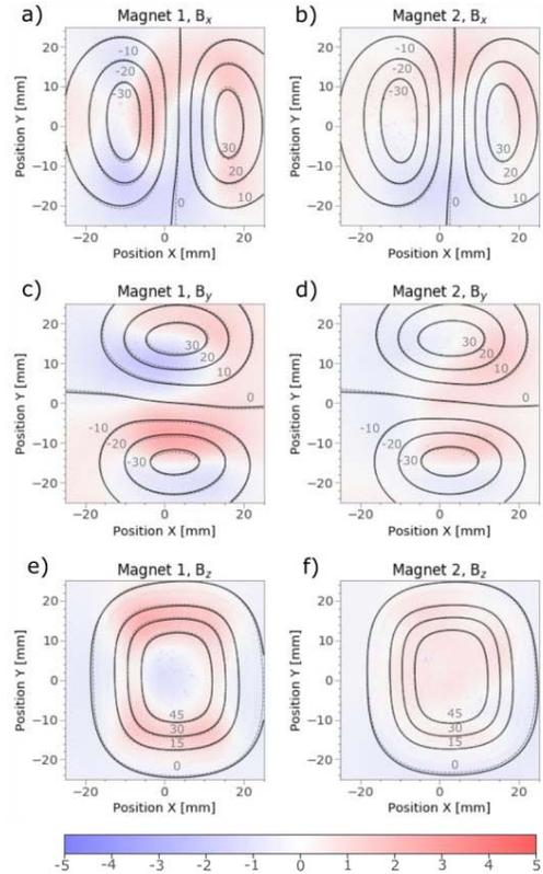
Figure 11. Magnetic field components of the two magnet samples after the first mechanical manipulation step
