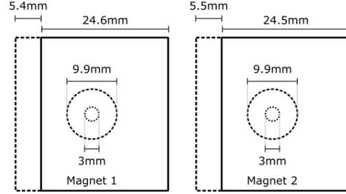
Figure 7. Sketch of the measured dimensions after the manipulations
