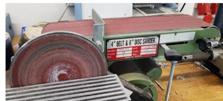
Figure 4. Sandpaper machine used for final polishing of the magnets
