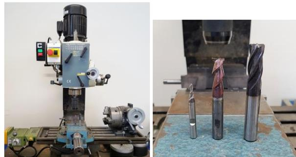
Figure 3. (a) Milling machine used to manipulate the magnets; (b) Specific tools used to perform the drills and cuts
