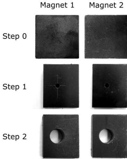
Figure 6. Mechanical manipulation steps of two sample magnets
