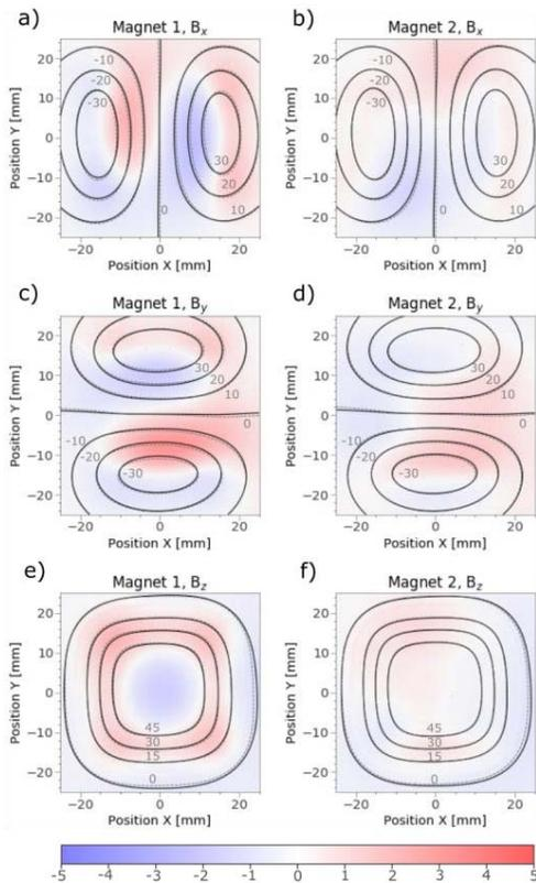
Figure 10. Magnetic field components of the two original magnet samples
