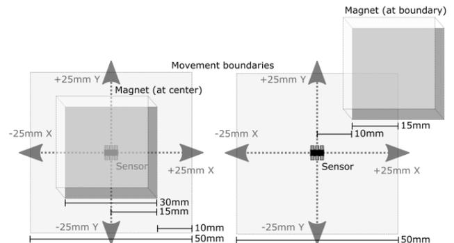
Figure 8. (a) Sketch of the experiment layout with the magnet centered over the sensor; (b) Representation of the magnet positioned over one of the extremities of the boundaries
