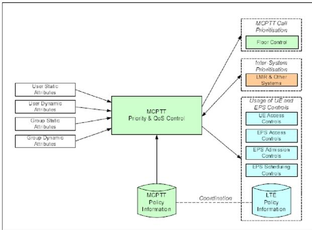
Figure 6. A conceptual on-network MCPTT priority model
