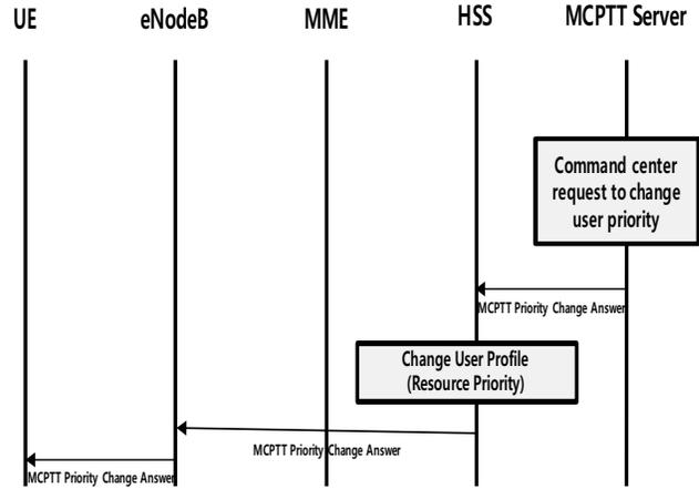
Figure 10. Command center request to change priority procedure
