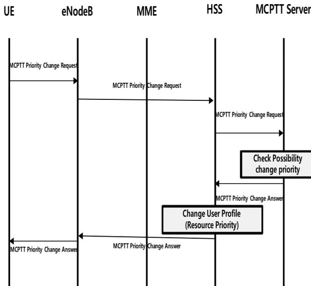
Figure 9. MCPTT user request to change priority procedure
