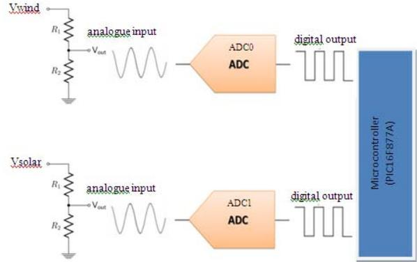
Figure 3. Solar - Wind Self - Intervention using ADC channel of PIC16F877A Microcontroller.
