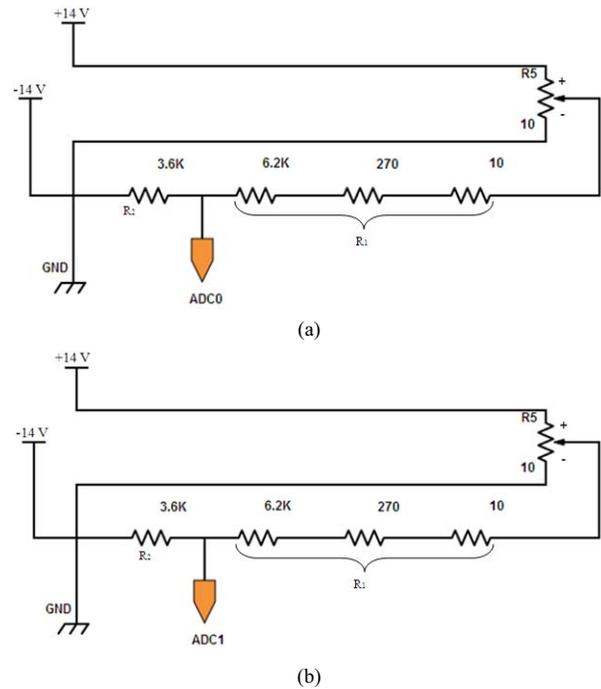
Figure 2. Solar – Wind Voltage Divider Circuits – Voltage - Base.
