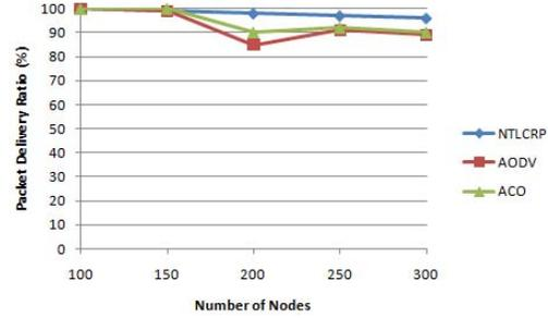
Figure 9. Comparison of packet delivery ratio in different number of nodes
