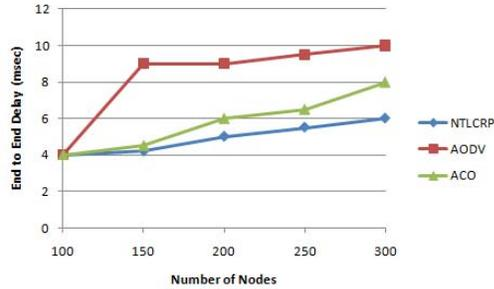
Figure 11. Comparison of end-to-end delay in different number of nodes
