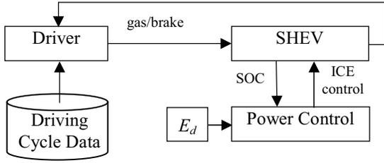
Figure 2. Configuration and components of the whole system.
