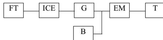
Figure 1. Configuration and components of SHEVs [24].
