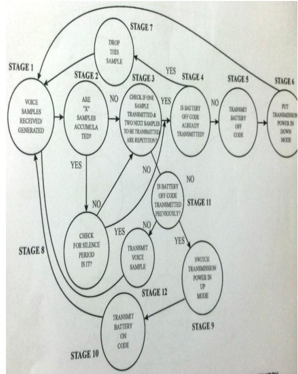
Fig. 2. State Transition Diagram for Signal Generation and Transmission at Mobile Station.[8]
