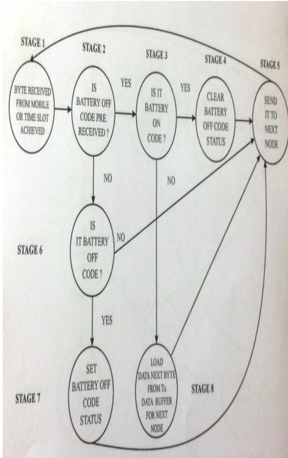
Fig. 3 State Transition Diagram for Interleaved Signal Transmission to Next Node (BTS) Received from Mobile Station at a Local Node (BTS).[8]
