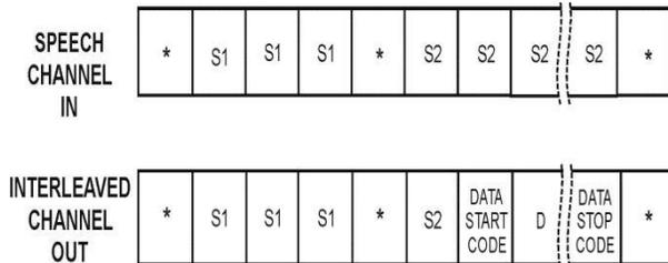
Fig. 1. Philosophy of Data Interleaving Symbols: S1, S2= Repetitive Speech Bytes\*= Speech Byte (S) D= Data Byte (S) [8]
